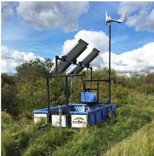
In the fall of 2015 the LSWC solar and wind powered watering system was on demo with a producer along the South Heart River. Systems like this are a cost effective and low maintenance way to provide off stream water sources for livestock.
